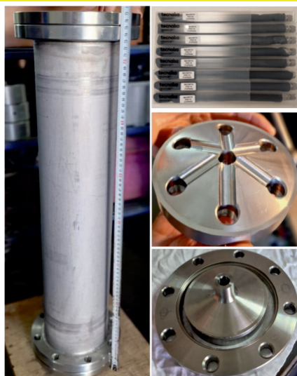
Membrane separator for hydrogen removal
