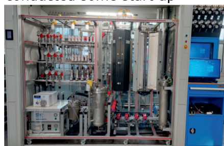
Propane dehydrogenation unit
